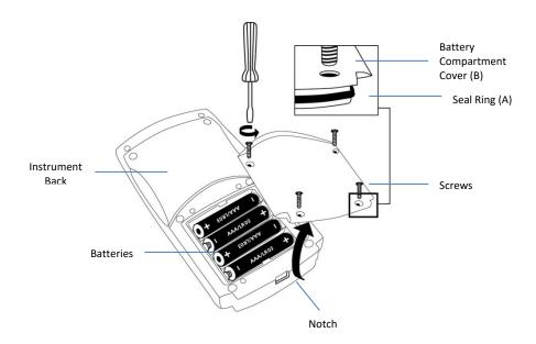
To ensure that the instrument is waterproof:
